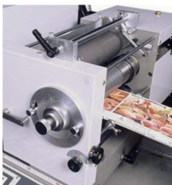
▲ Cool UV flexo varnish coating station (V)
