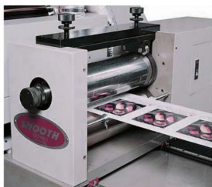
▲ Magnetic rotary die cut station (R)
